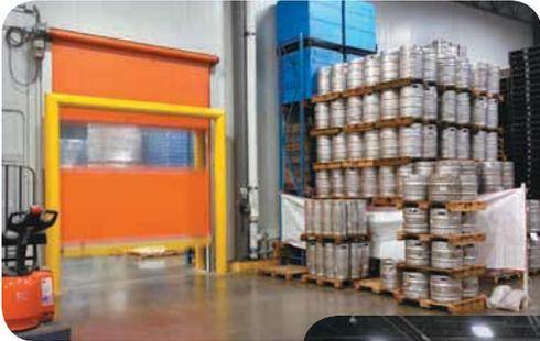
**DOORS:** One of the major improvements C&L made was to the warehouse doors its semi trucks use when loading and unloading beer and soda. The high-speed doors go up or down in eight seconds, about two to three times faster than an average garage door. The doors cost \$20,000 each and pay for themselves in seven to nine years.
